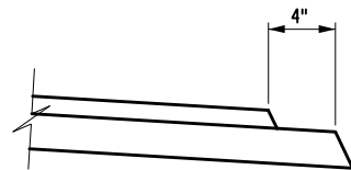
ASPHALT STEP DETAIL NOT TO SCALE
